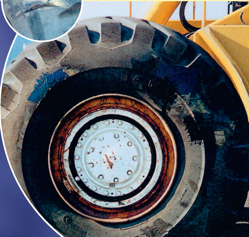
Front end loader tyre repaired using the '60' Durometer Paste Elastomer.
