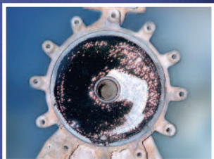
'80' Durometer Fluid Elastomer used to reconstruct the worn seam of a slurry pump.
