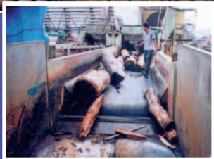
'60' Durometer Rapid Paste Elastomer used to carry out an instant repair on a conveyor belt at this log mill, which was back in service within 30 minutes.
